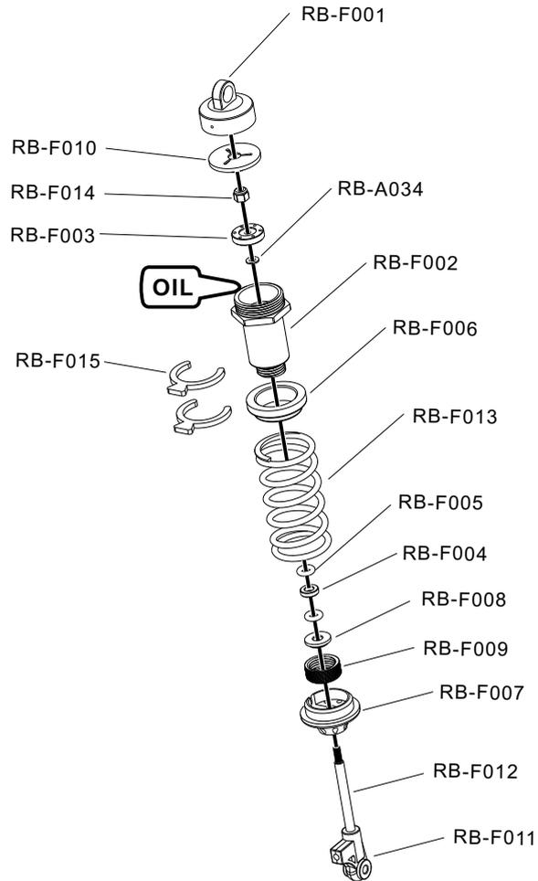
NOTE: The user could adjust the effect of the rear suspension according to different racing ground by instralling shock body spacer.
