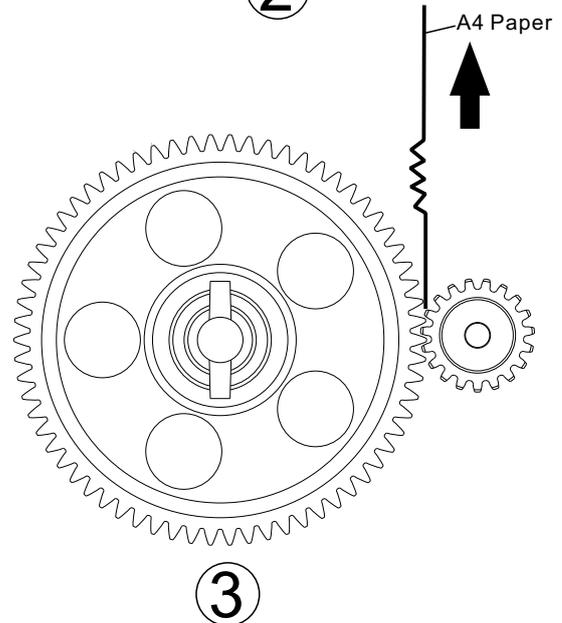
**Caution:** The space between the two gears should be the same thickness as one piece of A4 paper. We can put one piece of A4 paper between the two gears before assembly and take it away after finish.
